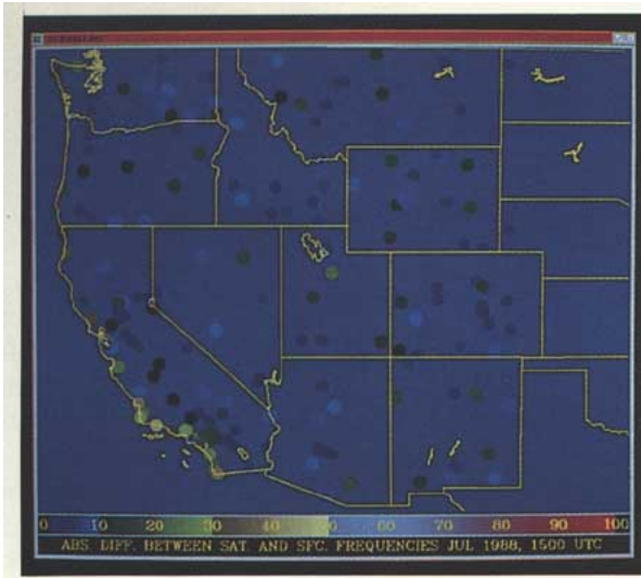
FIG. 7. Difference image. Colors represent the absolute difference (in percent cloud cover) between the satellite-derived cloud frequency and the frequency computed from surface observations (July 1988, 1500 UTC).
