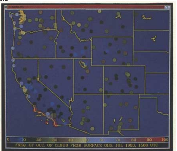
FIG. 6. Cloud frequency composite from surface observations for July 1988, 1500 UTC. Circles represent a 50-km diameter centered on the reporting station.
